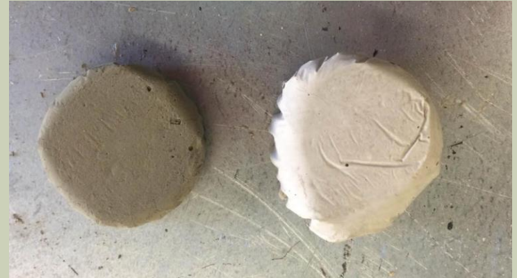
Fig 10: Cement & Fly Ash Samples for ASR
