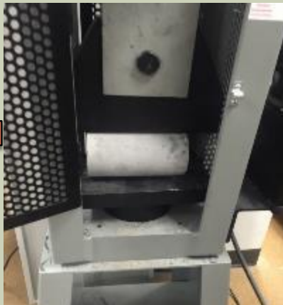
Running Tensile Strength Test
