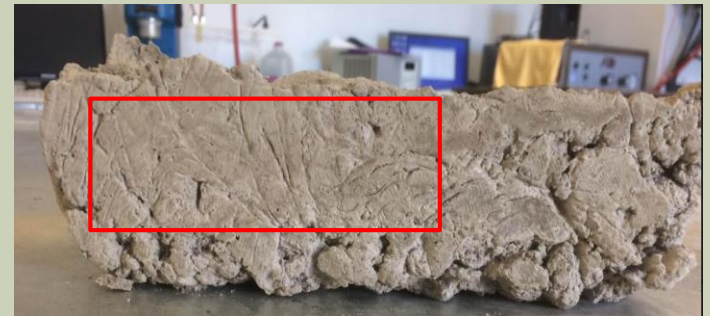
Fig 8: Side view Freeze-Thaw Sample
