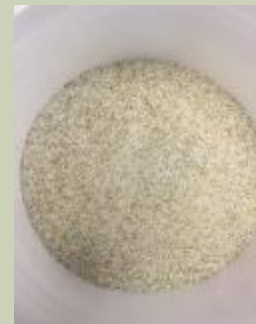
Fig 2: Recycled Glass-Sand (Coarse)
