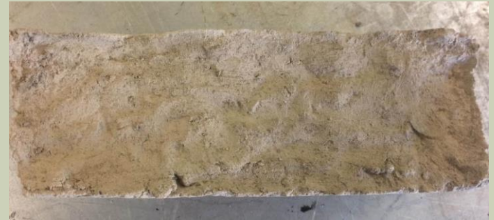
Fig 7: Top view Freeze-Thaw Sample
